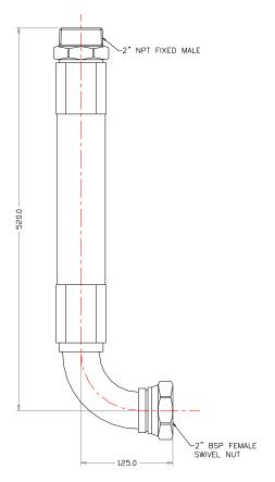
**Specification:** Hose Construction: Twin Steel wire Braided Oil Resistant
