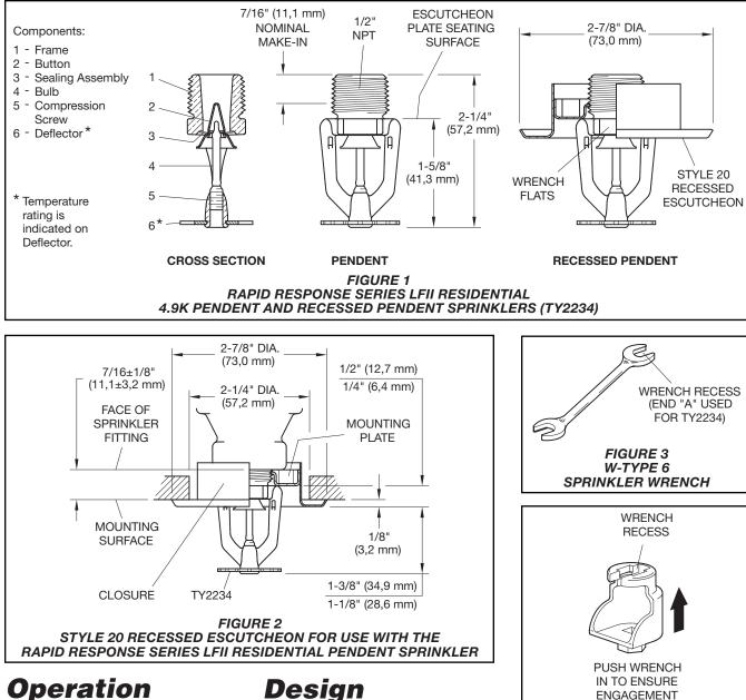
The glass bulb contains a fluid that expands when exposed to heat. When the rated temperature is reached, the fluid expands sufficiently to shatter the glass bulb, allowing the sprinkler to activate and flow water.
