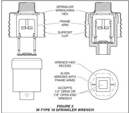
distort the sprinkler inlet with consequent leakage or impairment of the sprinkler.
