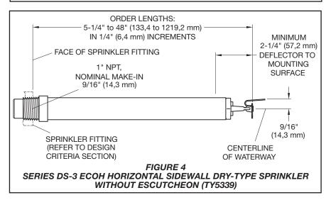
For wet pipe system installations of 1 inch NPT Series DS-3 Dry-Type Sprinklers connected to CPVC piping, use only the following TYCO CPVC fittings:
